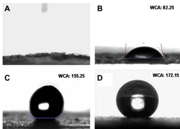
Figure 3. Water droplet (5 µL) images for cotton covered by SiO<sub>2</sub> nanoparticles (A), coated by silica hydrosols with subsequent HFTMS modification without heat treatment (B), coated by silica hydrosols with subsequent HFTMS modification and heat treatment at 100°C for 10 min (C), and coated by silica hydrosols with subsequent HFTMS modification and heat treatment at 150°C for 10 min (D).
