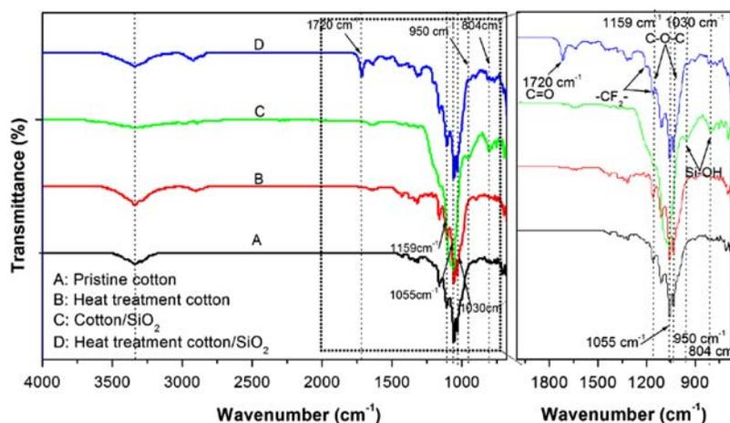
Figure 2. FT-IR spectra of pristine cotton (A), pristine cotton with heat treatment at 150°C for 10 min (B), cotton covered by SiO<sub>2</sub> nanoparticles with heat treatment at 150°C for 10 min (C), and the cotton fabric coated by the silica hydrosol followed by HFTMS modification and heat treatment at 150°C for 10 min (D).
